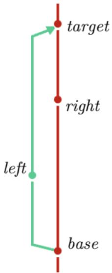
**Three-way merging:** integrate consistent changes introduced by the two branches.
