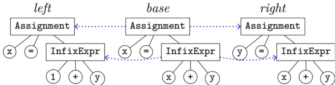
**AST matching:** When manipulating *base* AST into some variant, the matched two nodes (e.g. Assignments) are recognized as the same one.
