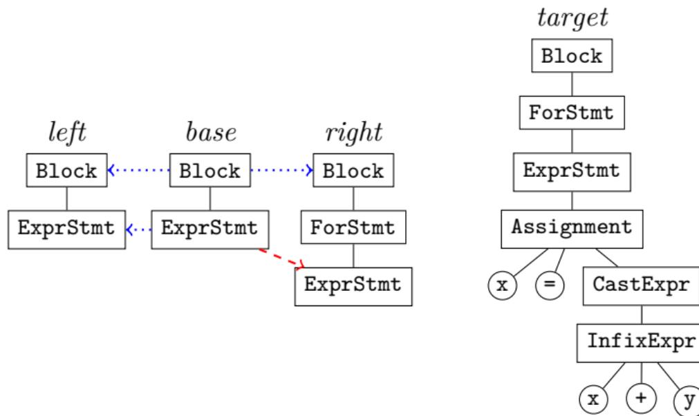
Shifted code in *right*: copy the subtree of ForStmt, and replace its child subtree (ExprStmt) with computed merged result.
