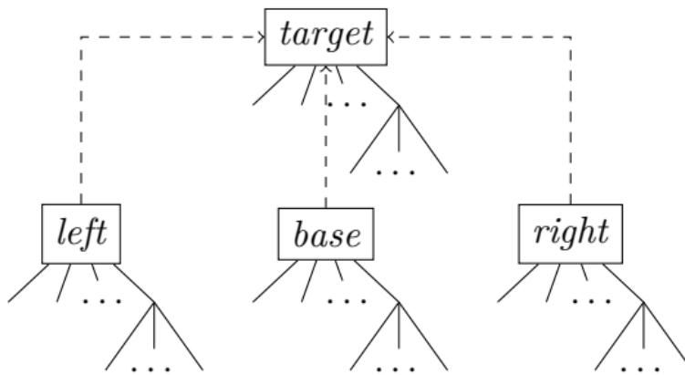
Structured merging recognizes source code as AST (abstract syntax tree), which has higher merge accuracy than unstructured merging.
